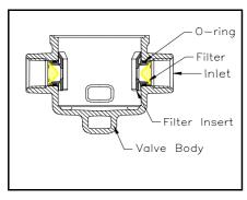
The filter screens are attached to an insert that is fitted into the valve body inlets. With the cartridge removed the 2 inserts and filter screens can be easily removed from the valve body.
