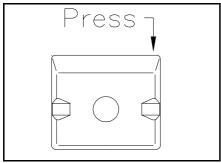
Remove the insert by pressing the top corner. This will rotate the insert allowing easy removal from the valve body.
