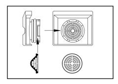
There is a place on either side of the filter insert where you can get your finger nail underneath the filter screen. By pulling the filter screen away from the insert it will "pop" out.
