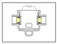
Place the insert back into the valve body, making sure the angled edge of the insert faces out.
